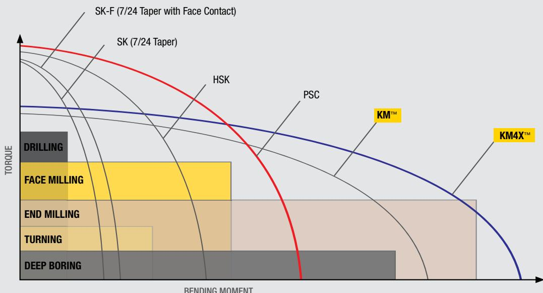
The Polygonal Shank Coupling (PSC) is an established ISO 26623 standard connection, offering modular flexibility and utility for lathe and multi-axis machine tool applications.
